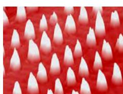
Magnetic cobalt nanodots on a reconstructed gold surface. The magnetic nanodots have a lateral separation of 7.4 nm, are 1 atom high and 4 nm in diameter. The hypothetical magnetic storage density is 10 Tbits / square inch.
