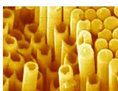
Polystyrene nanotubes (molecular weight 800000 g/mol) fabricated by wetting of porous templates. The nanotubes have wall thicknesses of 20 nm to 40 nm and lengths up to 100 µm.
