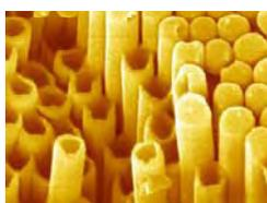
Polystyrene nanotubes (molecular weight 800000 g/mol) fabricated by wetting of porous templates. The nanotubes have wall thicknesses of 20 nm to 40 nm and lengths up to 100  $\mu\text{m}$ .
